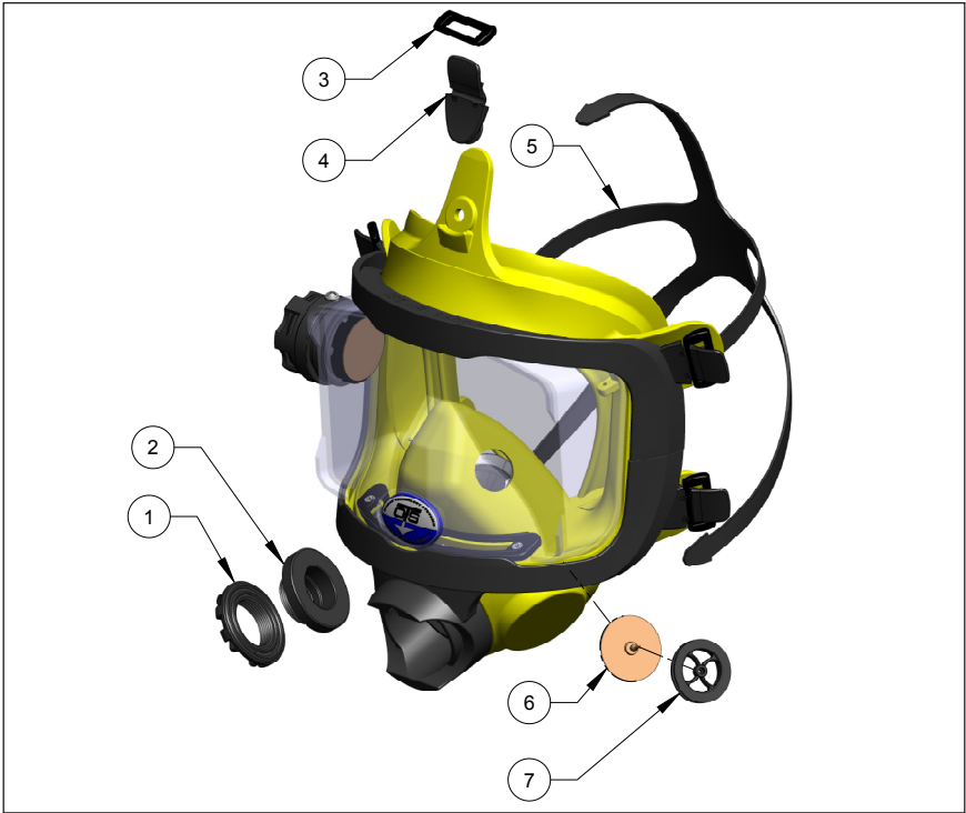
Figure 15: Guardian FFM Exploded View
