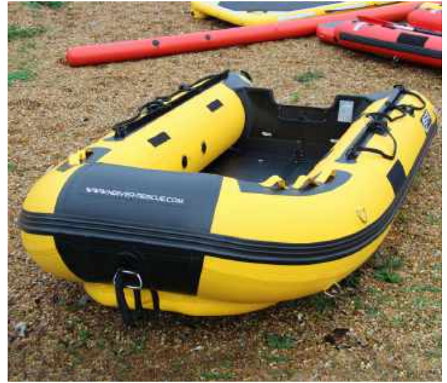
DS360 Commercial Inflatable with aluminium floor & stainless steel bow tow point
