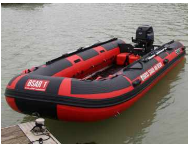
DS460 Commercial Inflatable with aluminium floor & stainless steel bow tow point
