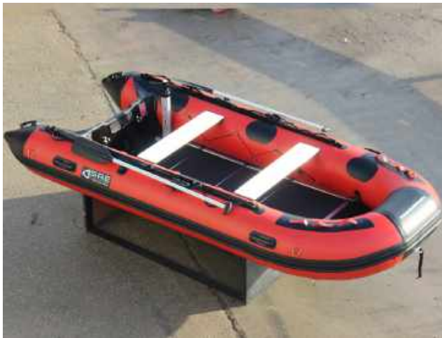
DS380 Commercial Inflatable with aluminium floor & stainless steel bow tow point
