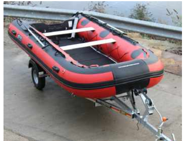
DS420 Commercial Inflatable with aluminium floor & stainless steel bow tow point
