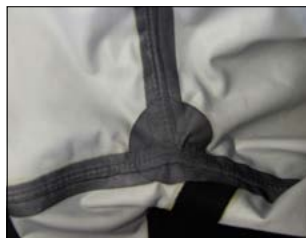
Internally taped and reinforced seams
