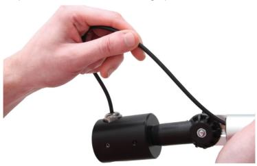
Step 4 - Attach the camera mount to the reach pole
